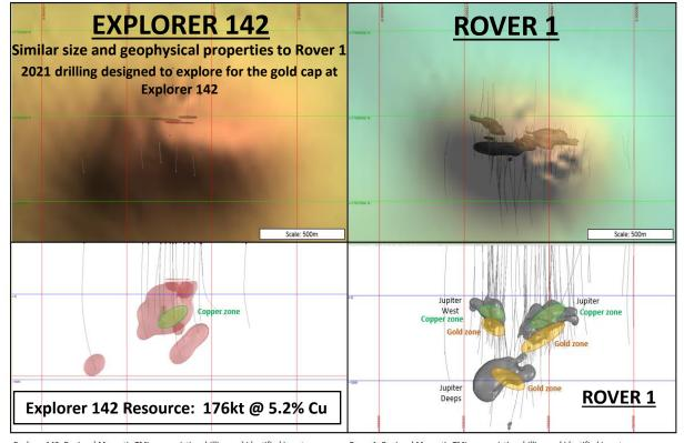
Explorer 142: Regional Magnetic TMI over existing drilling and identified ironstones The magnetic anomaly is of a similar size and intensity as Rover 1 Only a fraction of the ironstone has been identified to date. Ironstone is open to west and down dip. Gold rich 'root zone' to be discovered. Rover 1: Regional Magnetic TMI over existing drilling and identified ironstones Scaled to provide a direct comparison with Explorer 142 Rich gold zone in the 'root zone' of ironstones
