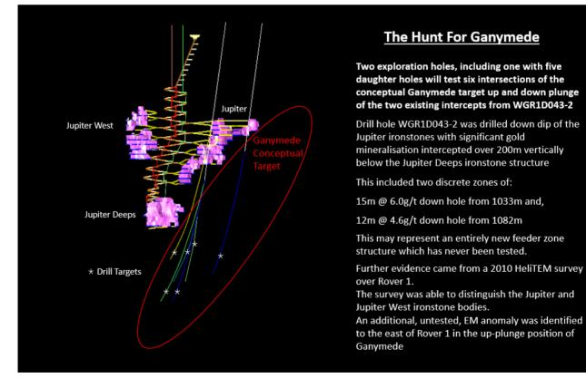
Two drillholes are designed to test the lateral up and down plunge mineralisation extents.
