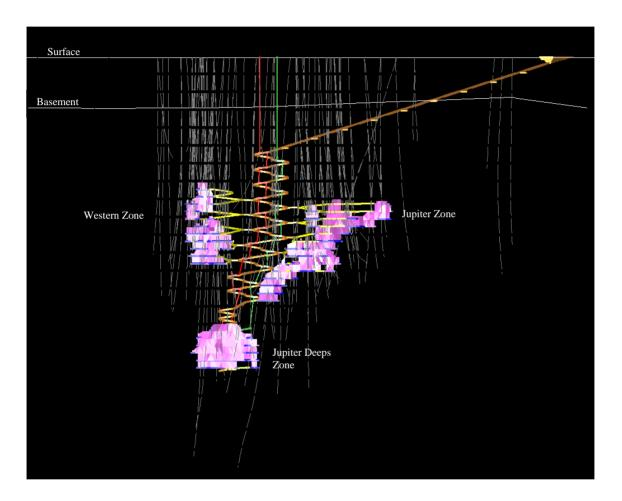
Figure 2: Rover 1 design option with the 85,000m of drilling coverage (grey lines) completed on Rover 1 by previous owners overlain. Capital development (brown), operating development (yellow) ore development (blue), stoping (purple), escapeway network (green) and ventilation network (red).
