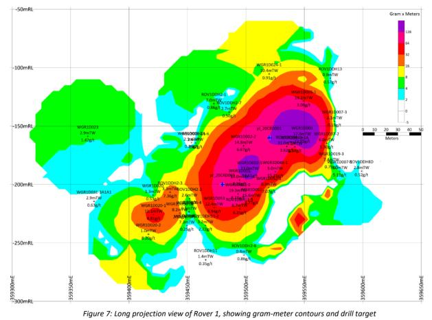
Figure 7: Long projection view of Rover 1, showing gram-meter contours and drill target
