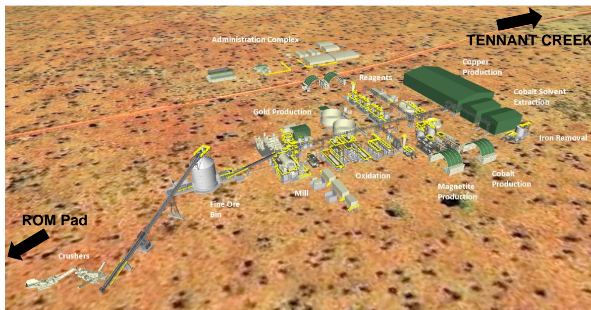
Figure 1: Representative layout of the Rover 1 Processing Plant
