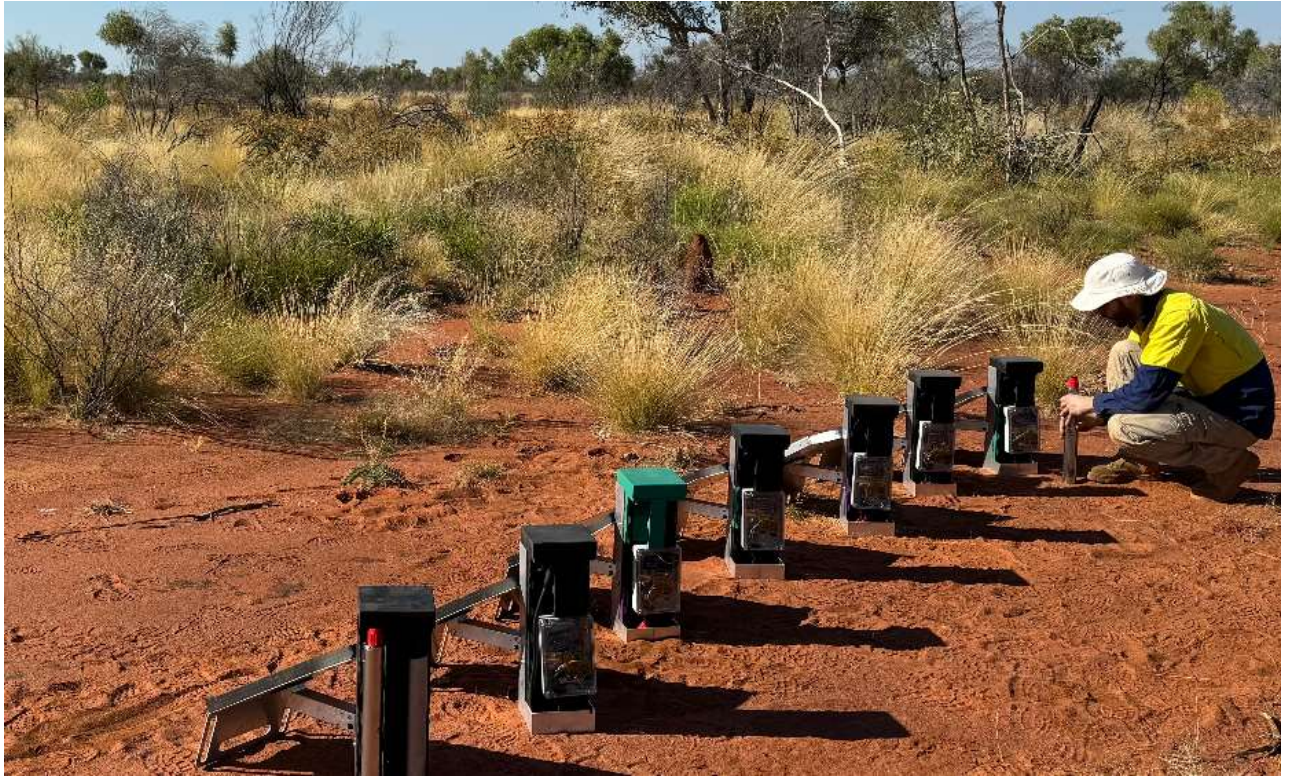
Figure 4: Ambient Noise Tomography sensors being prepared for deployment in the field. The seven sensors shown would each be spaced approximately 250m apart making a total line or “array” of 1.5kms for the survey.
