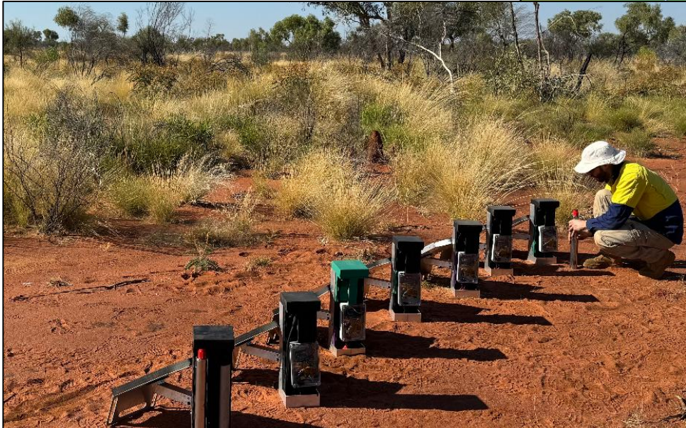
Ambient Noise Tomography sensors being prepared for deployment in the field. The seven sensors shown would each be spaced approximately 250m apart making a total line or "array" of 1.5kms for the survey.
