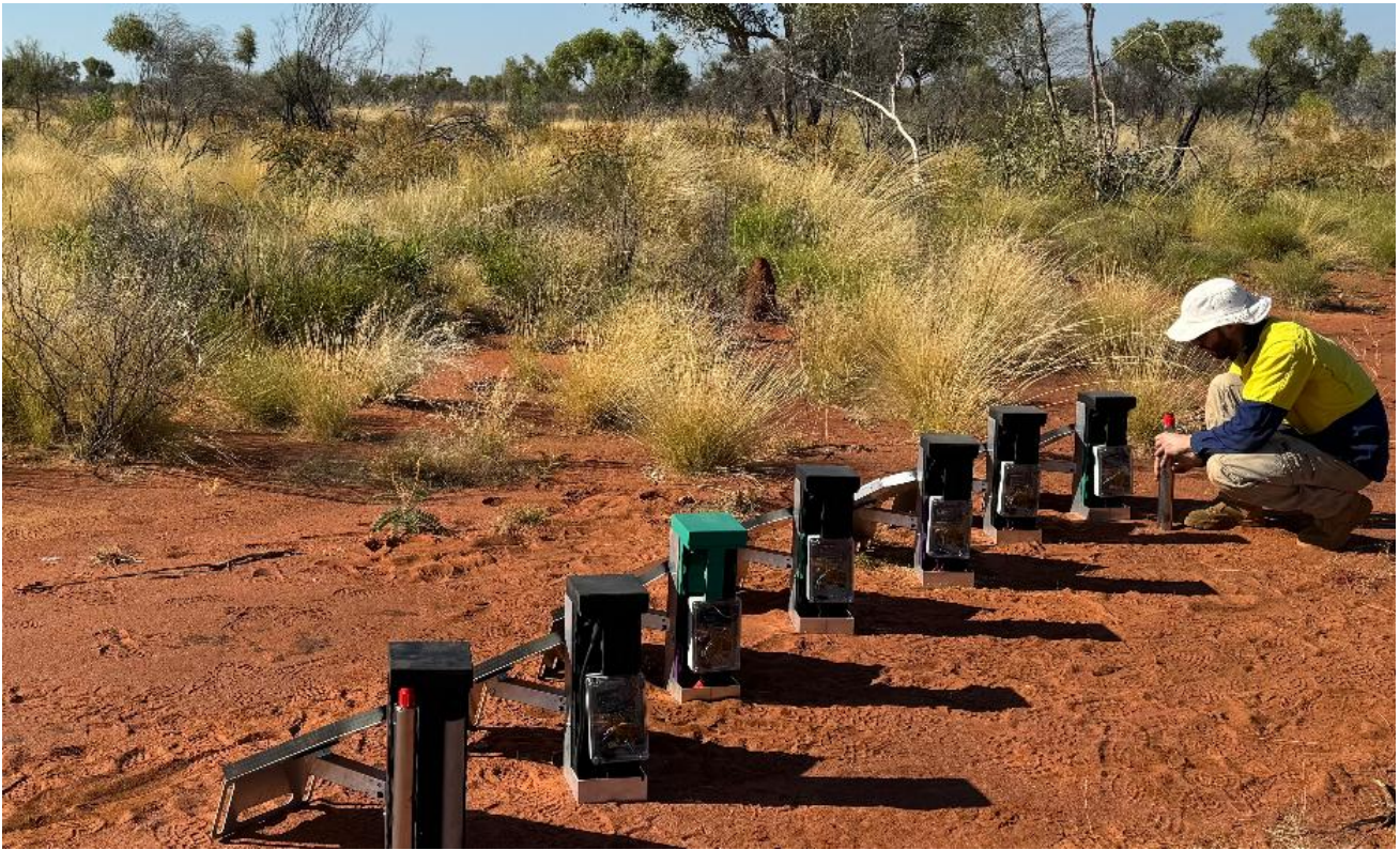
Figure 7 Ambient Noise Tomography sensors being prepared for deployment in the field.
