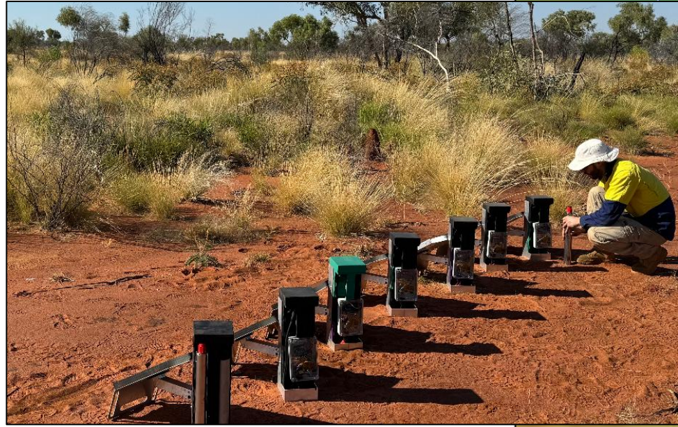
Ambient Noise Tomography sensors being prepared for deployment in the field. The seven sensors shown would each be spaced approximately 250m apart making a total line or "array" of 1.5kms for the survey.
